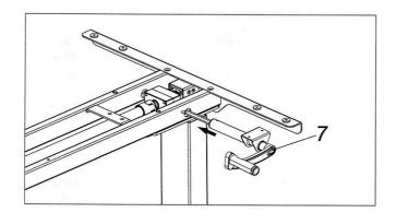
Option 2: Installed the handle on the left side of the table.
