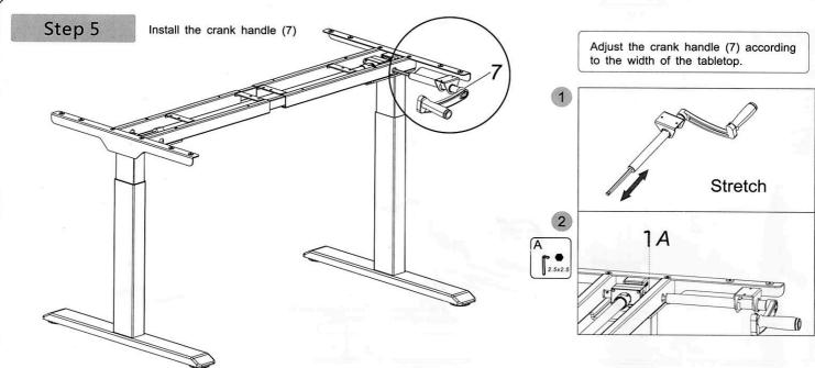
Option 1: Installed the handle on the right side of the table.
